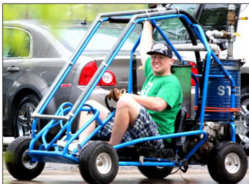
Green Go-kart: Mitch Sempowicz, a recent graduate of the Masters in Technology program, takes his biomass fueled go-kart for a spin. Sempowicz built the biomass gasifier for a class project.
