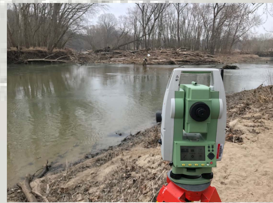
Figure 4. Survey of the site using the TS02 total station. Photo taken on March 12, 2018.
