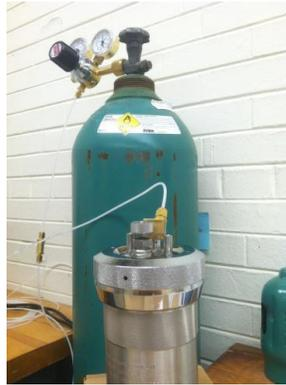
*Figure 3: Oxygen Filling*
