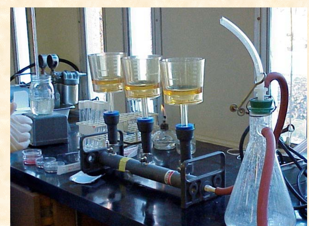
Manifold filtration system
