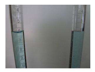
The scale divisions on a graduated cylinder are generally determined by its size. For example, the 50-mL graduated cylinder is divided into 1 mL increments. However, the scale of a 10-mL graduated cylinder is divided into 0.1 mL increments, and the scale of a 500-mL graduated cylinder is divided into 5 mL increments.
