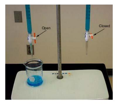
Burets are available in a limited range of sizes; the most common size is 50-mL. The scale of a 50-mL buret is divided into 0.1 mL increments. Therefore, when the liquid level in a buret is read, it is read and recorded to the nearest 0.01 mL. Water or aqueous solutions are the most common liquids used with a buret, and, if made the buret is made from glass, the bottom of the meniscus is taken as the liquid level.
