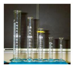
The volume of liquid in a graduated cylinder is obtained directly by reading the calibrated scale. In most situations, the liquid will be water or an aqueous solution.
